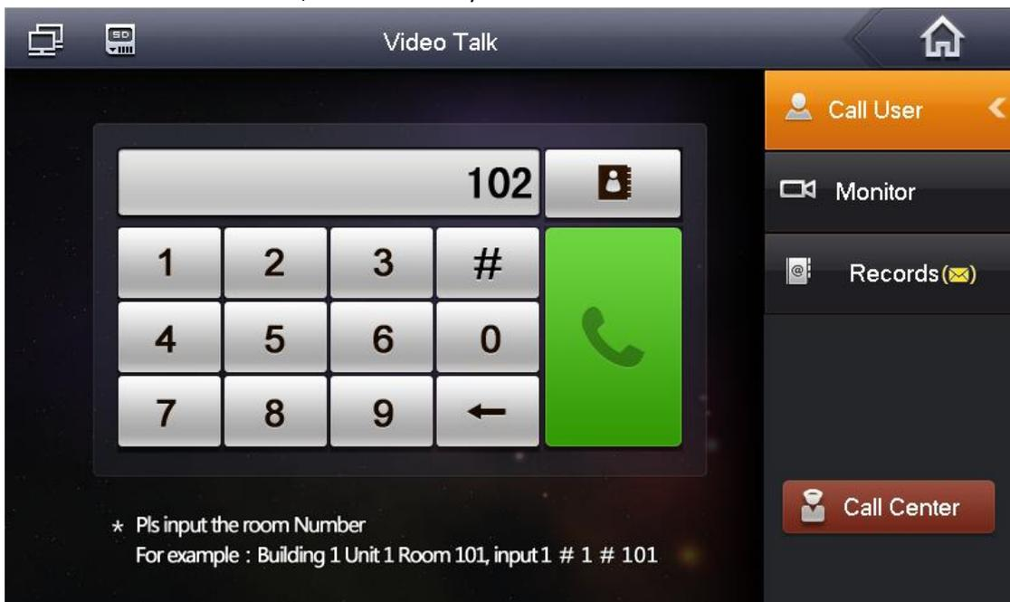
When calling VTH in different Units, dial the Room Number. Such as when calling from 101 in 01#02 to 102 in 02#02, dial 02#02#102 directly.
